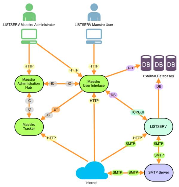
The arrows between the components indicate the direction of communication and the bubbles at the arrow heads indicate the port that is used for this communication. Note, that sometimes the communication goes in both directions (requiring an open port on both sides) and sometimes it only goes in one direction.
